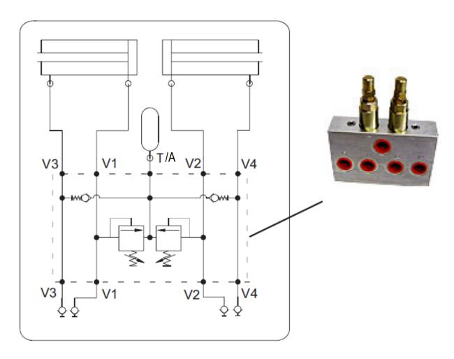
Figure 3. 4- and 5-hose hydraulics
