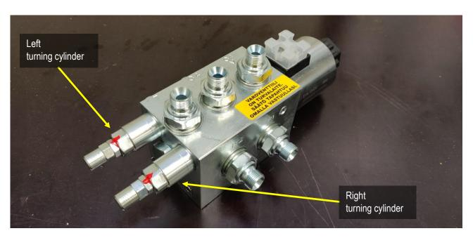
Picture 33. Relief valves of 6/2 -electric valve and double relief valve
