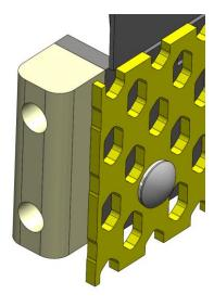
Picture 24. M20 washer is added under the bolt
