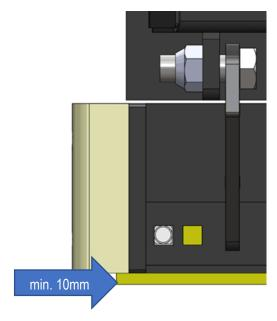
Picture 23. Minimum distance of the blade edge from the blade frame
