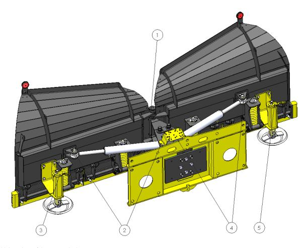
Picture 31. Locations of the grease nipples
