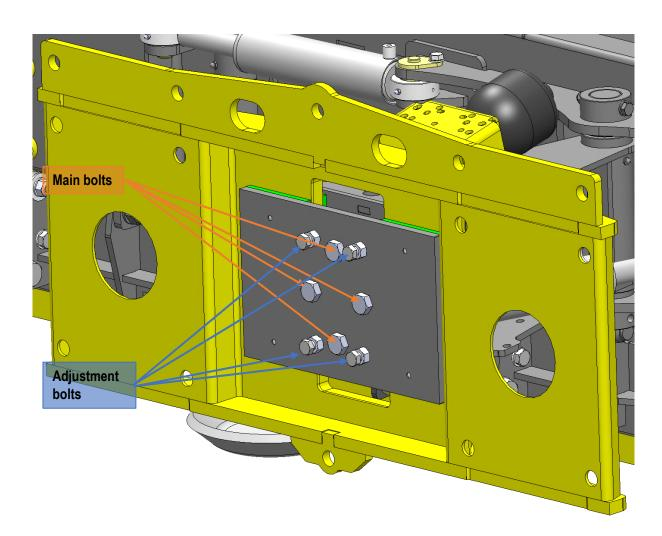
Picture 20. Adjusting flotation
