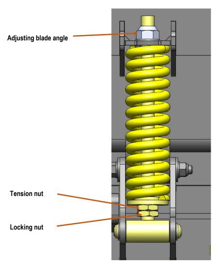
Picture 19. Adjusting the spring
