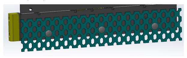
Picture 26. Perforated blade after it has been lowered
