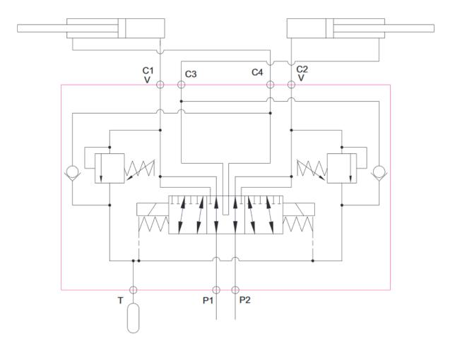
Figure 3. Diagonal valve circuit diagram.
