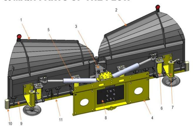
Picture 2. Main parts of the plow
