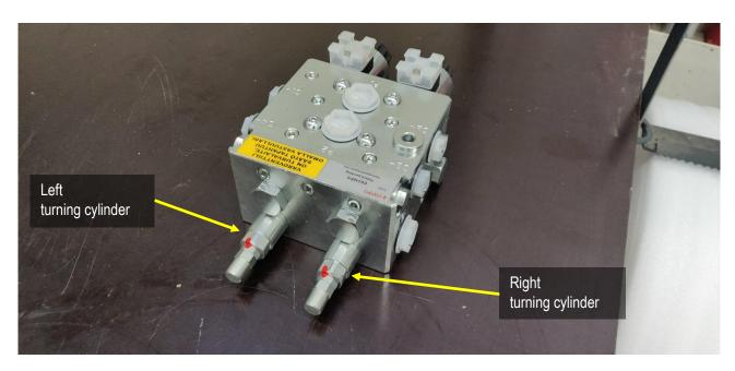
Picture 34. Relief valves of 8/4 -electric valve
