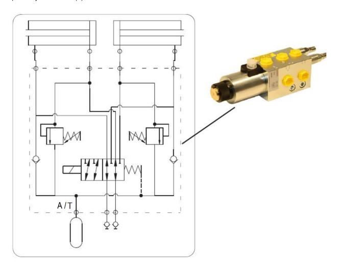
Figure 2. 2- and 3-hose hydraulics
