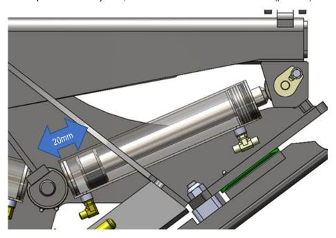
Picture 4. Cylinder piston is at the bottom in extreme positions
