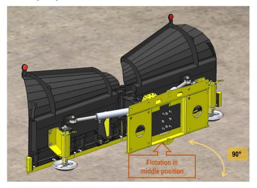
Picture 3. Optimal position for plowing, flotation in middle position and plow perpendicular to the ground
