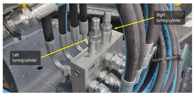
Picture 32. 5-hose hydraulics relief valves
