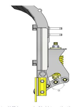
Picture 14. Minimum  $\alpha\text{-angle}$  of the joints must be at least  $5^\circ$
