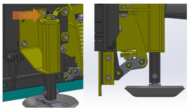
Picture 21. Adjustment handle of the support leg
