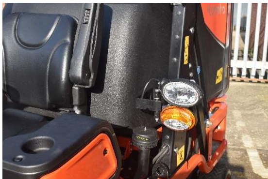
Side mounted lighting
