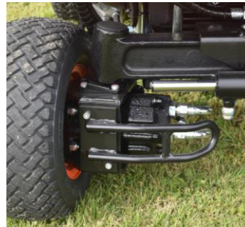
Rear axle. Dedicated drive motors to each wheel.
