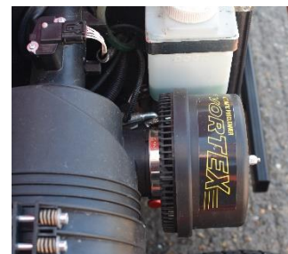
Vortex pre-cleaner removes the heavy dust and debris
