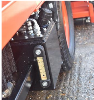
Visual check of the hydraulic oil tank level
